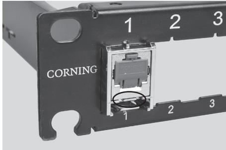
5. To remove jack from adapter release latch in the front and pull jack to the back
