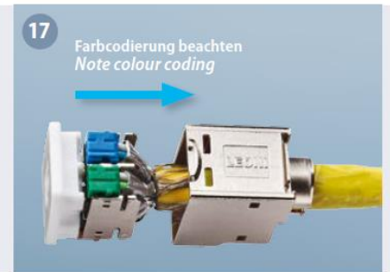
17 Wire Manager mittels Verpresshilfe in Gehäuse schieben. Push wire manager with the fitup-aid into the housing.
