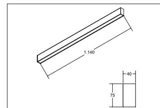
LED-Anbauprofil BIRO40, white, rectangular Lamp holder: LED, Mounting method: Surface mounting, Place of installation: Ceiling-mounted, Material: Aluminium / Acrylic, Degree of protection: according to DIN EN 60529 IP20, Protection class: (EN 61140) I, Voltage: 230V AC 50Hz, Power: 31.4W, Luminous flux: 2.430lm, Colour temperature: 3000 K, Light colour : White, Beam angle: 80°, Adjustability: Not adjustable, With control gear: Yes.
